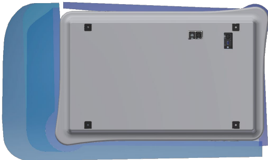
Figure 2 Protective fields of MiR100 and MiR200 when driving in reverse.
