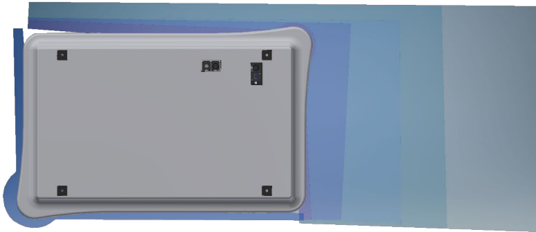
Figure 1 Protective fields of MiR100 and MiR200 when driving forward.
